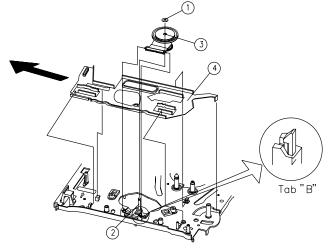
Fig.3-21 REEL GEAR TOTAL ASS'Y & CONNECT PLATE REMOVAL
